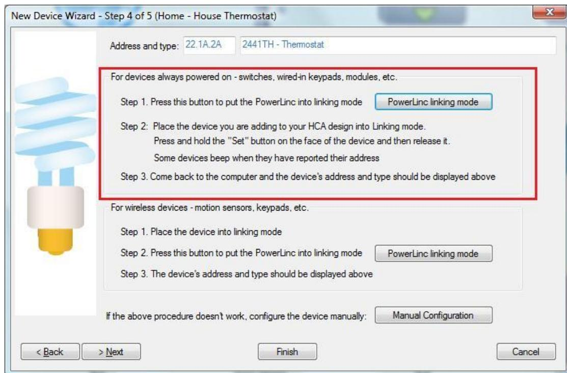
After the thermostat is added to your design choose the linking tab and link it to HCA. Several commands are sent to the thermostat to configure to report status as it changes.
