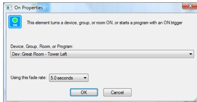
In this example the UPB device is told to turn ON with a 5 second fade rate. The fade rate can also be specified when using the OFF and DIM elements.
