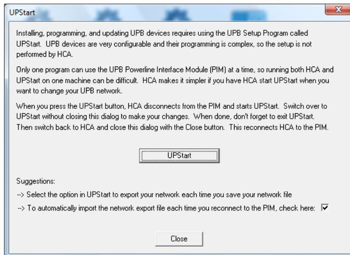
Press the UPStart button. At this point, HCA relinquishes its control of the PIM, then UPStart starts and its main window appears on your screen. Use UPStart to make your network and device modifications and when done, exit UPStart with File - Exit. Since in the first step above you selected the “Auto Export on File Save”, by exiting UPStart you are automatically saving and exporting your UPB network. Then switch back to HCA and close this dialog with the Close button.
