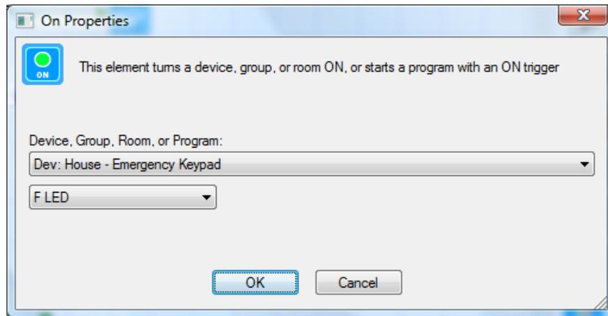
In this example, the Library Keypad F indicator is turned ON. To turn it OFF, the OFF Visual Programmer element can be used.
