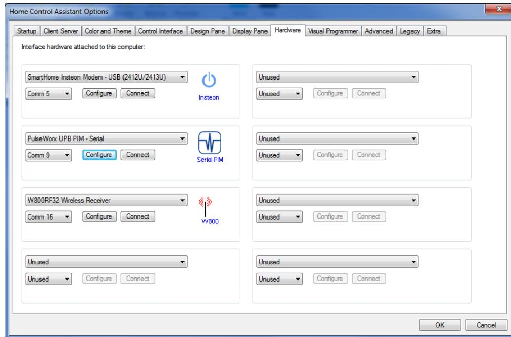
In the same way you identify all automation interfaces to HCA, all you need do is to select the interface type, communications port, and then press the **Connect** button. If HCA can read information from the PIM it displays a success message. Any problems with connection are noted in a failure message.
